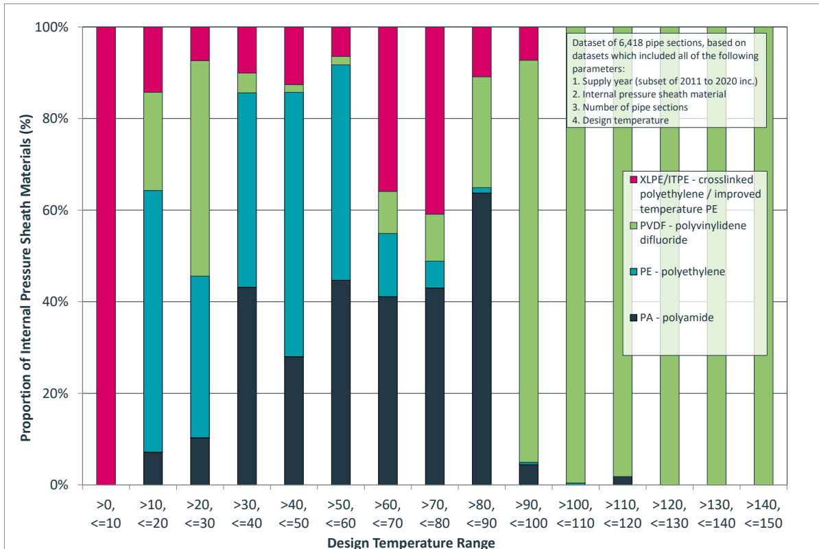
Figure 3.16 Internal Pressure Sheath Material per Design Temperature Range (last 10 years only)
